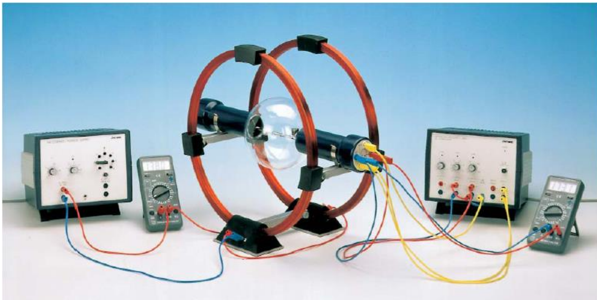
Fig.1. Experimental setup - By varying the magnetic field (current) and the velocity of the electrons (acceleration and focussing voltage), the radius of the orbit can be adjusted, such that it coincides with the radius defined by the luminous traces.
