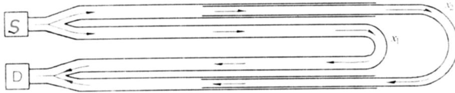
Figure 25-1: Interference scheme for acoustic waves reaching detector via two different routes; S – sound source, D – detector.
